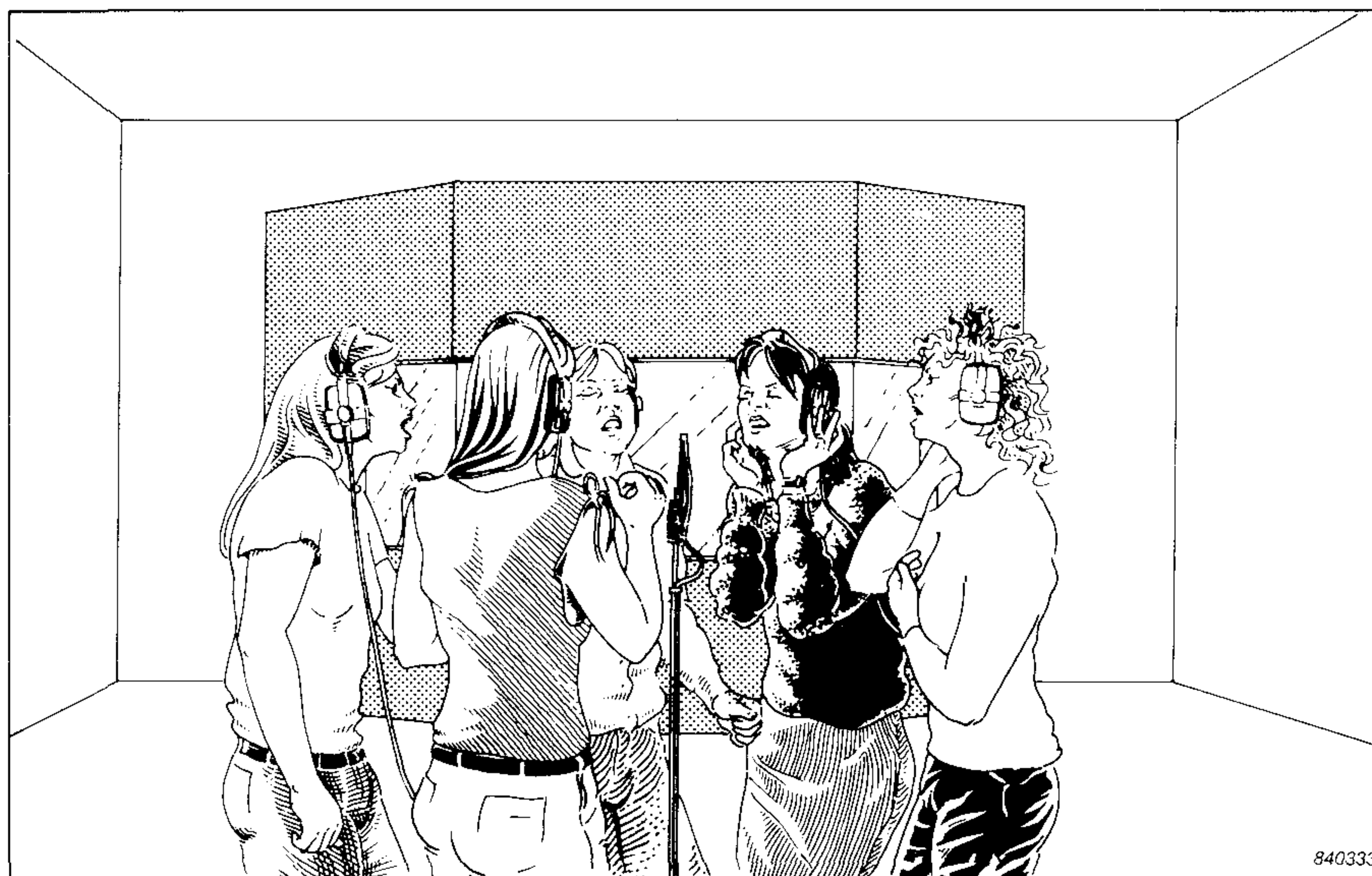
Fig. 2. A group of background vocalists encircling a B&K 4004 solves any problems about being on the "right side" of a mic's polar pattern
